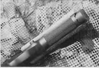
(left) The GRP II's lanyard mount is "buried" into the checkered steel mainspring housing totally out of the way until you need it. (right) Perfect machine checkering abounds on the front strap of the GRP II and the pistol's exterior surface is devoid of sharp edges.
